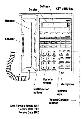
Press KEY MENU to display softkey names. This example shows the softkey names for the normal display.
