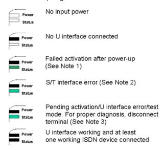
Note 1: For .5 seconds the STATUS indicator flashes quickly (8Hz)
