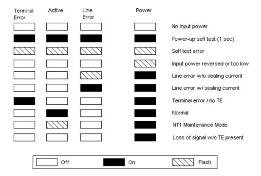
Any status display other than those shown above indicates improper NT1 operation. Push the reset switch or, if no improvement is obtained, refer to AT&T Practice 533-700-100.
