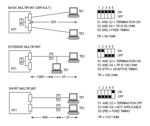
Note: Distances specified above are for 24-guage inside wiring cable and two terminals. These distances may vary for other cable gauges and different number of terminals. For additional details refer to the AT&T Practice 533-700-100.
